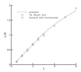
**Figure 4.** Flow past a circular cylinder for Re = 550: separation length versus t
