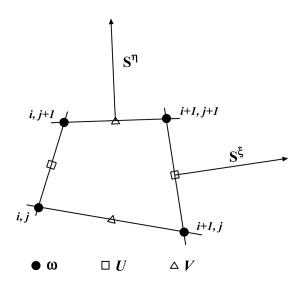
**Figure 1.** Elementary finite volume
