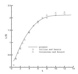
Dennis (1973). The experimental data of Coutanceau and Bouard (1977) are also given for completeness. The time evolution of the separation length for Re = 550 is shown in Figure 4 together with the numerical results of Loc (1980) and the experimental data of Bouard and Coutanceau (1980). In both cases, the present solutions are in good agreement with both the aforementioned numerical and experimental results.
