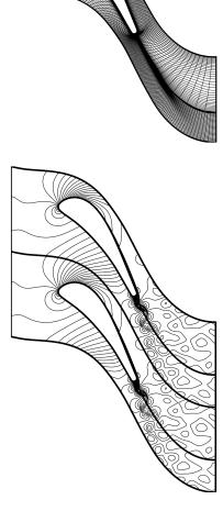
Figure 7. Mach number contours on the finest grid  $(\Delta M = 0.02)$
