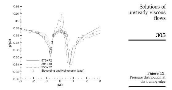
versus the curvilinear abscissa of Figure 5. The computed results show a clear trend toward grid convergence, and the line corresponding to the fine grid agrees quite well with the experimental data. It is noteworthy that the maximum difference between the experimental data and the fine-grid solution is about 1 per cent of the inlet total pressure. The space averaged value of the base pressure between  $s/D=\pm0.4$  is equal to 0.8847 versus the experimental value equal to 0.885.
